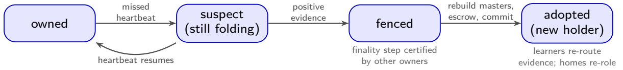
Figure 7. Membership state machines. (a) A joining node hydrates from relay state, trains in quarantine without contributing until every lane is current, and ramps its contribution after admission. (b) An owner that misses heartbeats is marked suspect and keeps folding while alive; once its loss is confirmed, its expert block is fenced at a certified finality step and adopted by a running learner that rebuilds the masters from the published experts.
